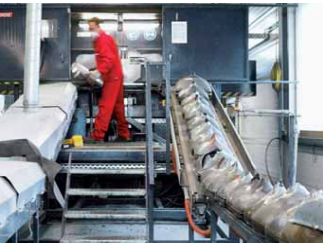
Waste at our dismantling centre is taken apart – to a certain extent by hand – and cleanly separated into individual fractions
